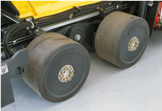
Pivoting front axle suspension for constant ground contact.
