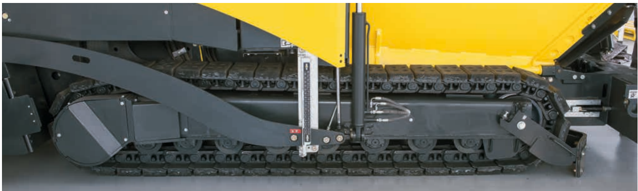
Individually controllable chains allow turning in the tightest of spaces.
