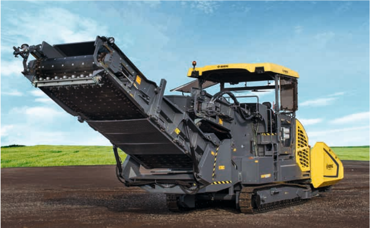
Speed: the conveyor belt can be changed fast thanks to quick release couplings.
