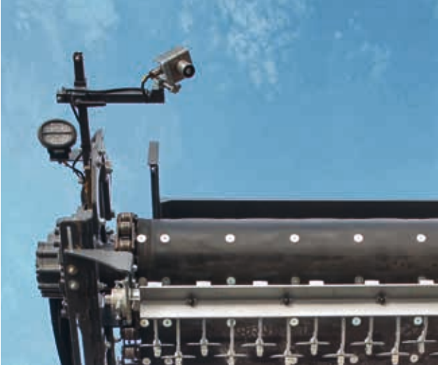
Automated material flow: the filling level sensor.
