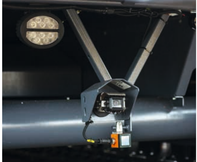
Synchronised speed: the distance sensor.
