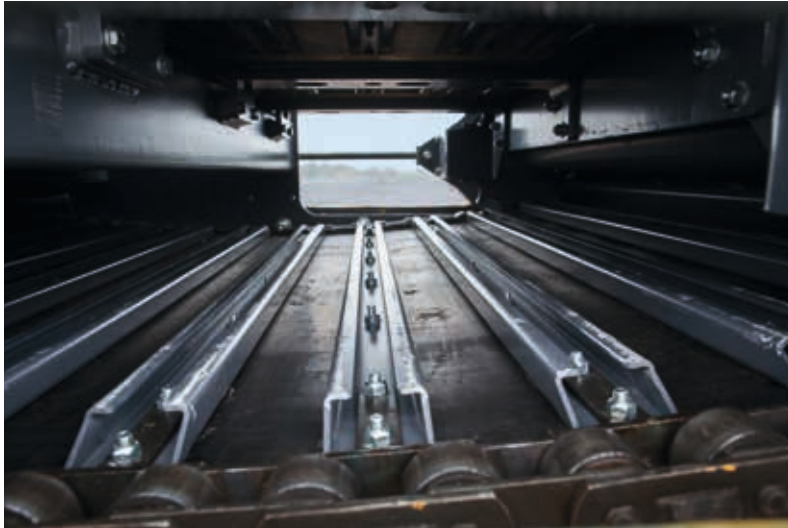
Reliability: the chain-reinforced conveyor belt.
