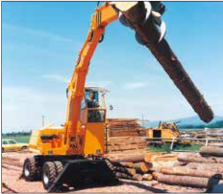
1974: Timber material handler with rigidly elevated operator's cab
