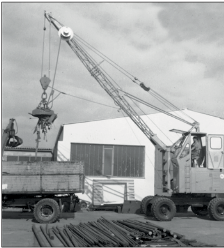
1962: rope-driven S833 with elevated operator cab
