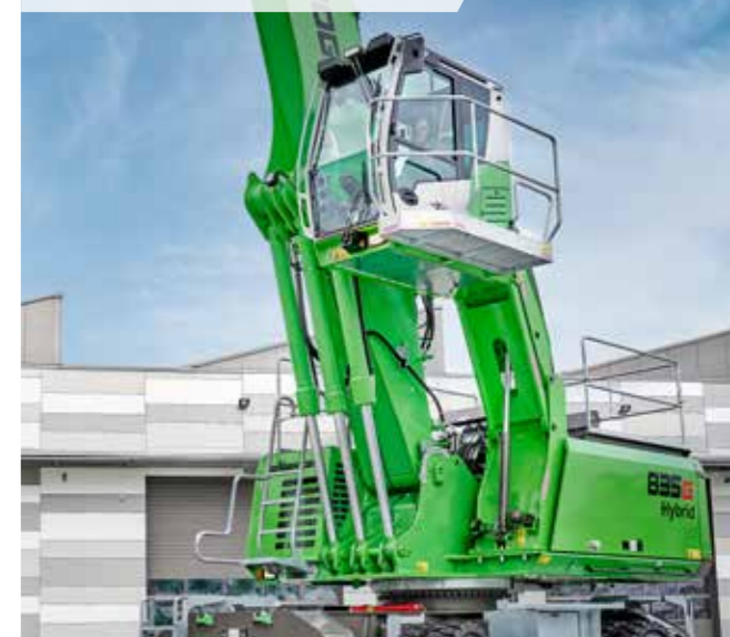
Particularly gentle movement of the cab thanks to cab elevation G280
