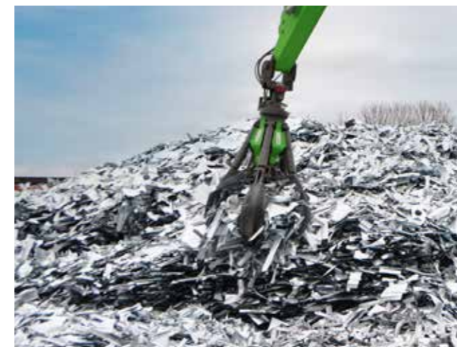
Orange peel grab (SGM), shell form half-open, for e.g. sheet metal waste
