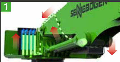
1 Boom lowers, gas compresses
