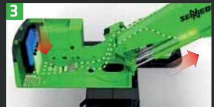
3 The nearly constant force transmission throughout the cylinder cycle supports the next boom lift
