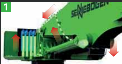
1 Boom lowers, gas compresses
